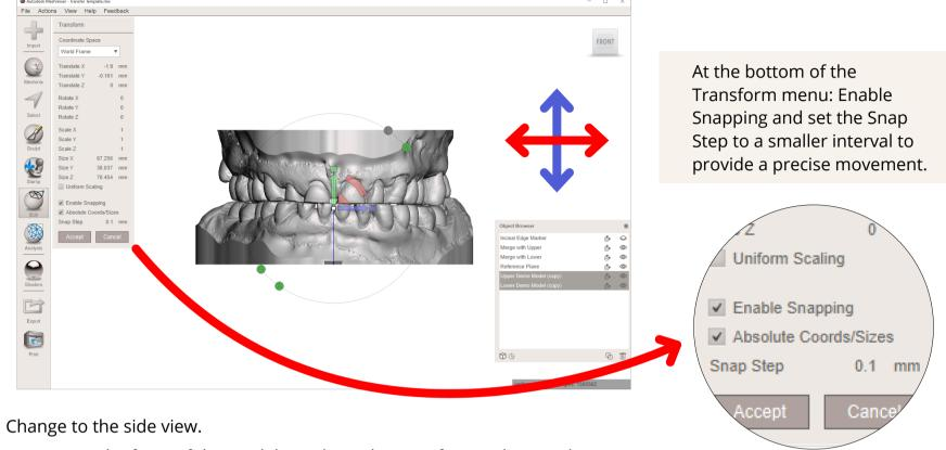
6. Zoom onto the front of the models, and use the transform to line up the
