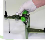
Position the magnet and retainer cup (supplied) over the magnetic base.
