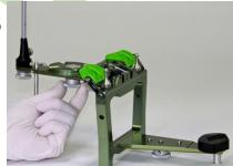
Tighten the mounting knob into the magnet retainer cup until snug, ensuring that the surface of the magnet sits flush with the magnetic base.
