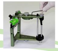
Tighten the allen screws into the magnetic base until snug.
