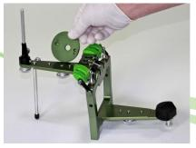
Position the magnetic base over the frame, noting the position of the index holes.
