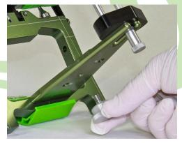
Remove the lower mounting plate knob from the articulator by pulling down on it while turning counter clockwise.
