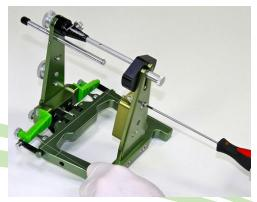
Attach the plate spacer to the lower articulator frame with the two allen screws.
