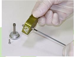
Remove the mounting knob and allen screws from the plate spacer.
