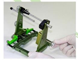
Thread the mounting knob supplied with the plate spacer thru the lower articulator frame and spacer plate.
