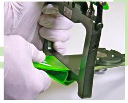
Raise the support leg up to secure the lower lip of the support leg against the articulator frame
