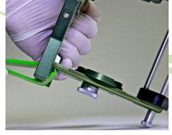
Place the support leg under the lower frame at rear, making sure the support leg lip "grabs" the lower frame
