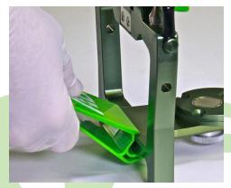
Release hand pressure on the support leg. It should now be attached to the articulator frame.
