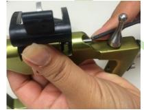
Push axis pin #1 back in so that it contacts and pushes out axis pin #2 from the opposite side. 8
