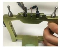
Using needle nose pliers, grip axis pin #1 where the spring was located and slide out of articulator with small pushes.
