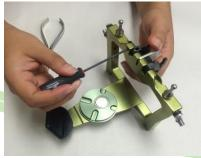
Using the 2.5mm hex screwdriver, loosen the two small allen screws on the front of the articulator.
