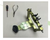
To remove and replace the latch, you'll need a 2.5mm hex driver and a pair of needle nose pliers (preferably curved).
