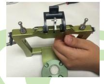
Axis pin #1 is now protruding and ready for removal.
