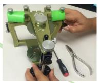
Place the articulator upper frame on the lower frame, ensuring that the steel centric plate fits in the slot on the upper frame. 18
