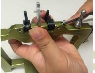
Push each axis pin thru the black centric latch and into the steel centric plate. Important: the two axis pins <u>must</u> meet in the middle of the steel centric plate.
