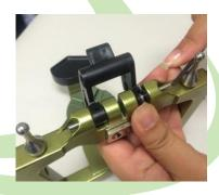
Slide the axis pin slowly thru the centric latch and spring combination.
