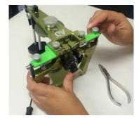
Insert the Dyna-Links pins in the left and right analogs and tighten the thumb screws on each one to secure them.
