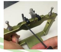
With both axis pins successfully installed, tighten the allen screws with the 2.5mm hex screwdriver.
