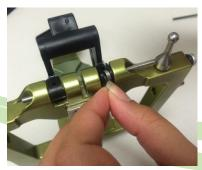
Place the return spring back into the centric latch, with the larger flat end of the spring against the articulator frame. 12
