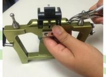
Using needle nose pliers, grip axis pin #1 and slide out of articulator.
