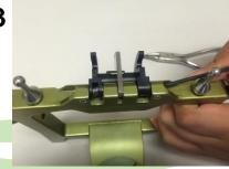
The black centric latch pivots on two axis pins. Using the hex screwdriver, push on the end of axis pin #2 until axis pin #1 protrudes from the opposite side.
