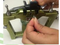
As axis pin #1 slides out, carefully hold spring so it does not get lost.
