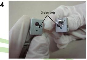
Ensure that the threaded portion of the hole on the lower clamp faces out (the lower clamp is threaded on one side only). On newer versions of the clamps, the small green dots (pictured above) will face each other when properly assembled.
