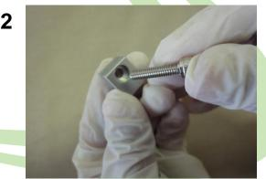
Insert the allen screw into the upper clamp. Note that the upper clamp has a large recessed area for the screw head to fit in.
