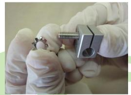
Place the lock washer over the screw (the washer will be between the upper and lower clamps when fully assembled).
