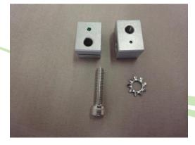
The four components of the toggle clamp assembly: the upper clamp, lower clamp, allen screw and lock washer.
