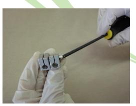
Screw the upper and lower clamps together. Do <u>not</u> firmly tighten the clamps until the bite fork and stem assembly are inserted.
